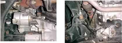
4. To remove the driver's side manifold. First remove the starter. Remove the driver's side manifold, studs and heat shields from the engine, through the top.
